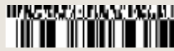
GS1 DataBar Composite combines 1D and 2D elements in a single bar code symbol
